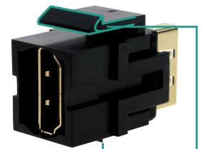
Step 1: Insert locking lug in cut-out and engage at the bottom Step 2: Snap the module into place at the top using the snap hook
