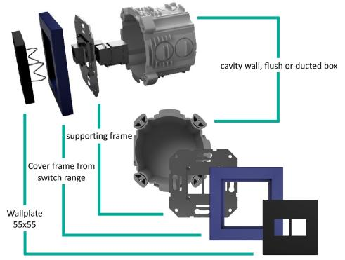
Due to the different module formats, the modules can also be integrated in cable ducts, base channels or room columns.
